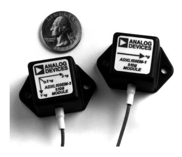
All that is required to use these modules is a +5 volt power supply. The module should be attached (i.e., screwed or glued down) securely to the object being measured, taking care that the axis of sensitivity, indicated by the large arrow on the top of the module, is aligned with the expected acceleration.
