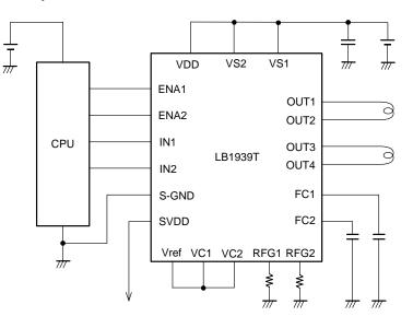
Constant current control mode: The RFG voltage is controlled so that Vref/4.5 = 0.2 V.
