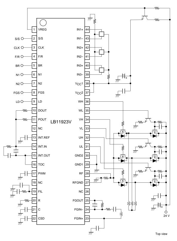
Sample Application Circuit 1 (P-channel + n-channel, Hall-effect sensor application)
