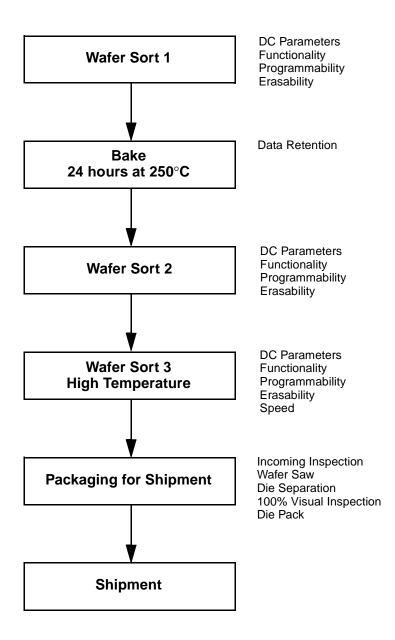
Figure 1. AMD KGD Product Test Flow
