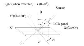
Light (when transmitted )  $Y(\varnothing\!\!=\!\!0^\circ)$   $(\theta\!\!=\!\!90^\circ)$
