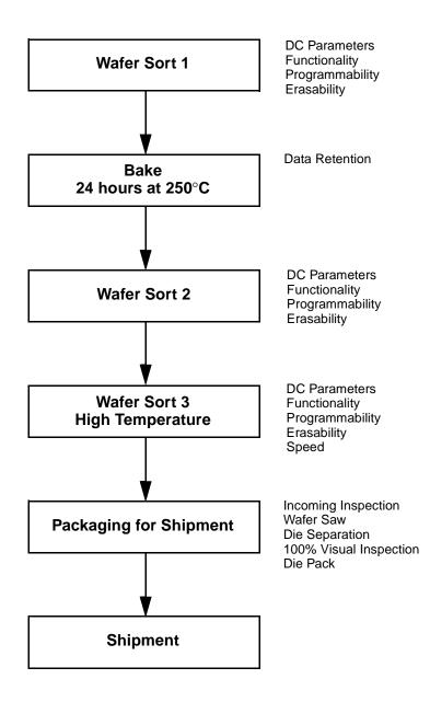
Figure 1. AMD KGD Product Test Flow
