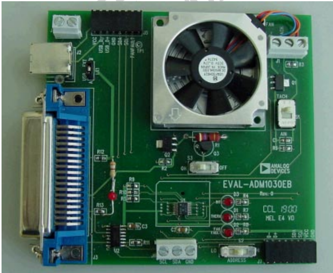
Figure2. ADM1030 Evaluation Board Picture
