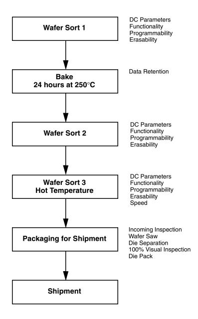
Figure 1. AMD KGD Product Test Flow
