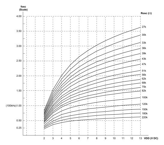
The recommended oscillator frequency is  $f_{OSCD}$  (decoder)  $\cong 50 \; f_{OSCE}$  (HT12E encoder)  $\cong \frac{1}{3} \; f_{OSCE} \; (\text{HT12A encoder}).$
