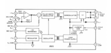
In data acquisition and control systems, the 2B23 may act as an isolated interface between the D/A converter output of a microcomputer analog I/O and standard 4 to 20mA or 0 to 20mA analog loops. In process control systems, the 2B23 may be used as a current output stage of a proportional controller to interface devices such as current-to-position converters and current-to-pneumatic transducers.
