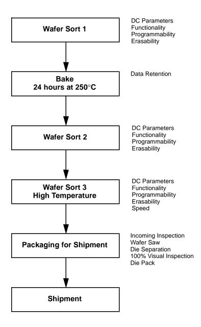
Figure 1. AMD KGD Product Test Flow
