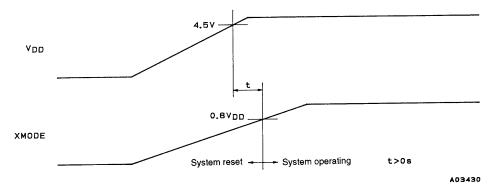
After application of power, the system will be reset if the XMODE pin is set low again.
