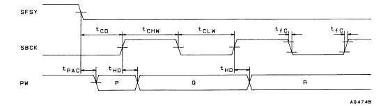
The LC8904Q subcode interface uses the user bit subcode sync word and start bit for system timing extraction. Therefore, since SBSY and SFSY will change with that timing, user bit transmission must follow the table shown below when using the values of  $t_{BW}$ ,  $t_F$ ,  $t_{CHW}$ ,  $t_{CLW}$ , and  $t_{CD}$  with the specifications listed in the preceding tables.
