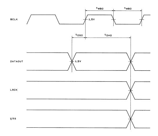
Note: When the validity fag is output from the DOUT/V pin.
