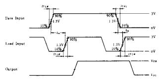
Input pulse: t<sub>TLH</sub>, t<sub>THL</sub> \le 10ns, PRR=1MHz, Duty cycle \le 50%
