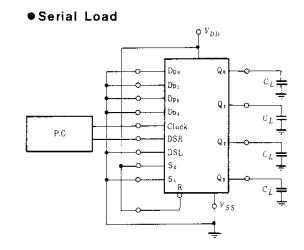
Interchange DSR with DSL and  $S_0$  with  $S_1$  for testing shift left.
