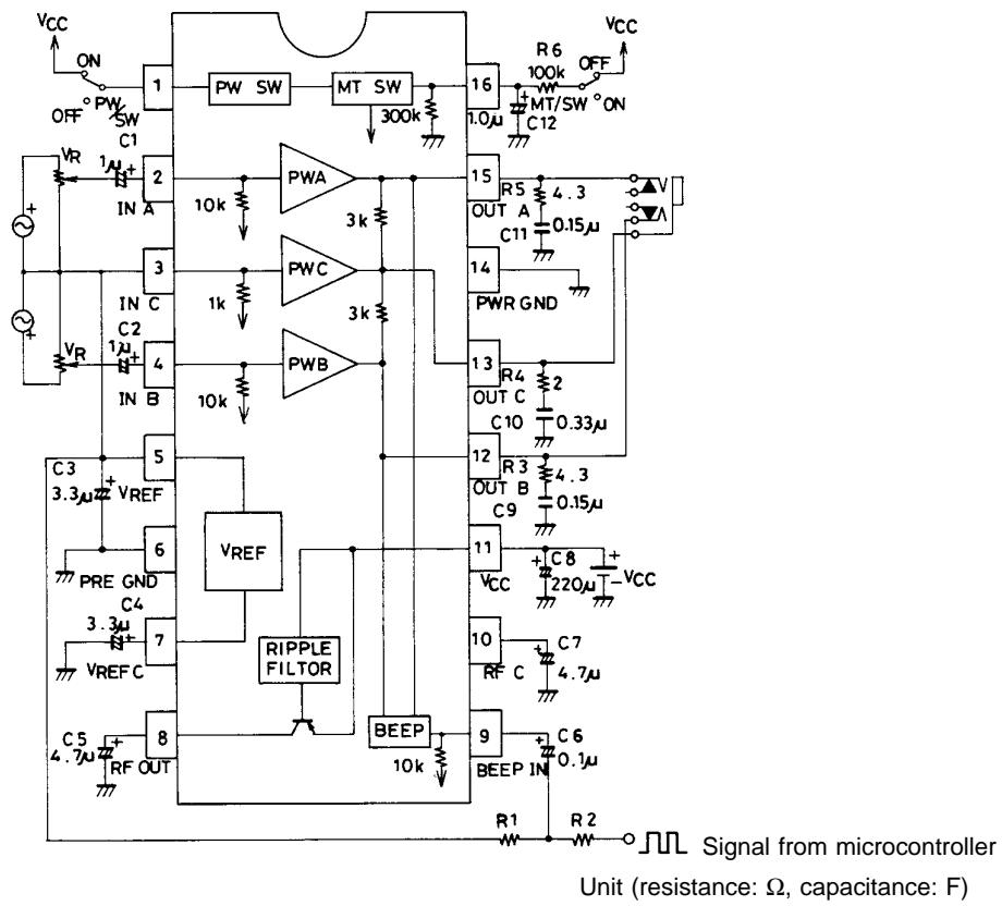
Unit (resistance:  $\Omega$ , capacitance:  $\mu\text{F}$ )
