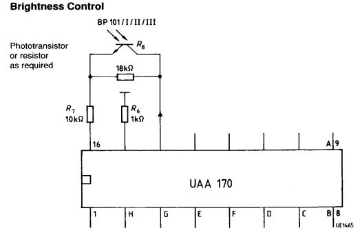
Pins 14, 15, and 16 serve to determine the diode current. Corresponding to the desired light intensity, the forward current of the diodes is linearly variable in the range Ir approx. 0 to 50 mA. The resistance at pin 15 defines the adjusting range. The resistances between pin 14 and 16 determine the current.
