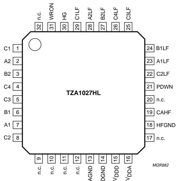
Fig.2 Pin configuration.
