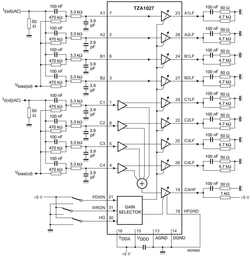
Fig.3 Test diagram.
