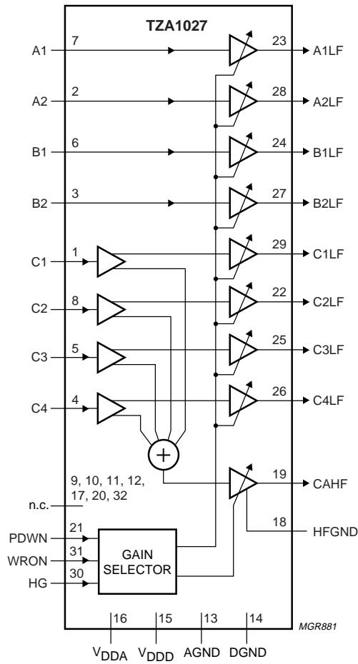
Fig.1 Block diagram.
