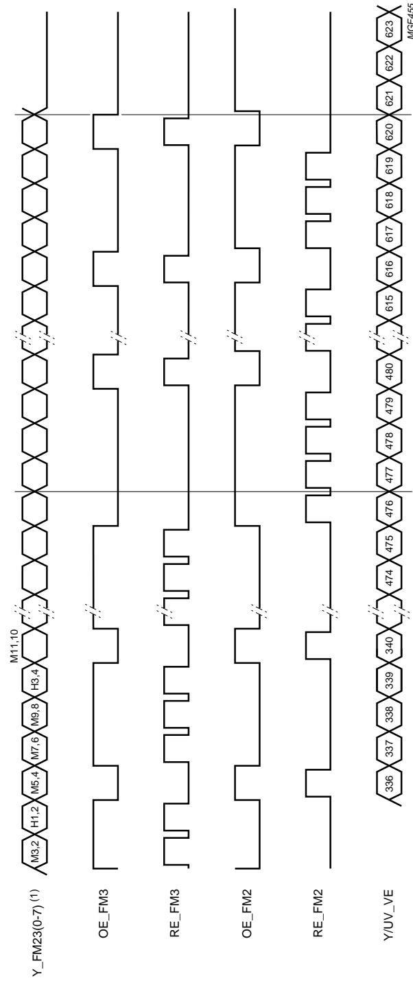
Fig.14 Line read timing FM2/3 FILM mode, second field.
