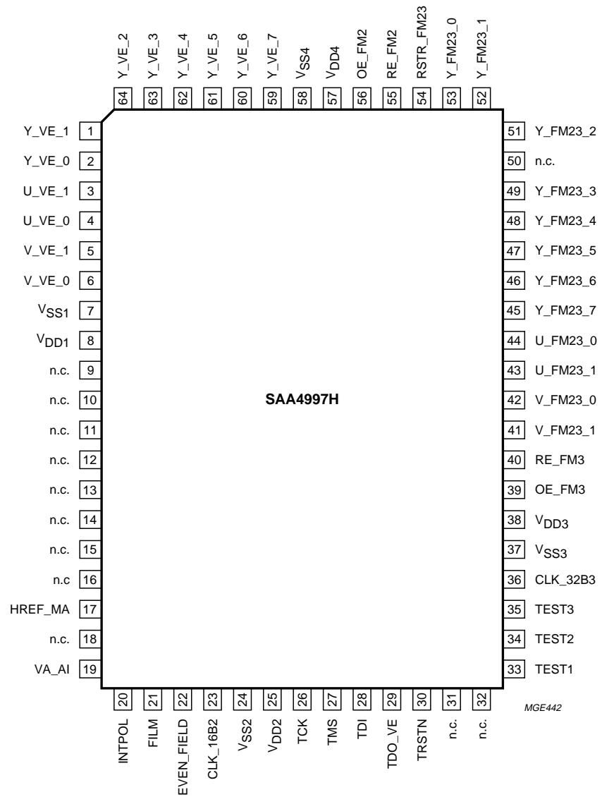
Fig.3 Pin configuration.
