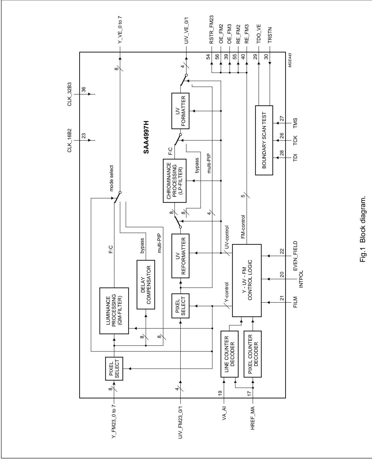
Fig.1 Block diagram.
