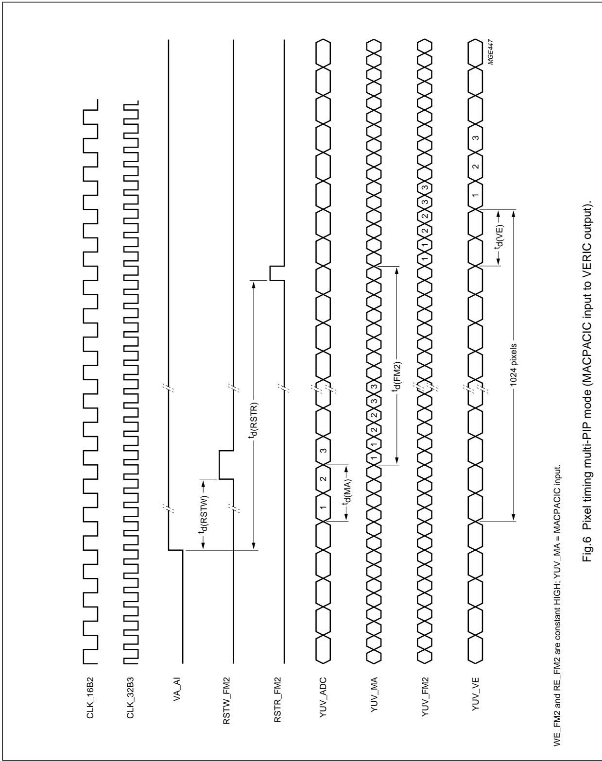
Fig.6 Pixel timing multi-PIP mode (MACPACIC input to VERIC output).
