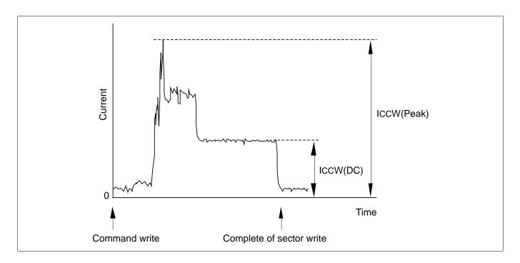
AC Characteristics (Ta = 0 to +60°C,  $V_{CC}$  = 5 V  $\pm$  10%,  $V_{CC}$  = 3.3 V  $\pm$ 5%)
