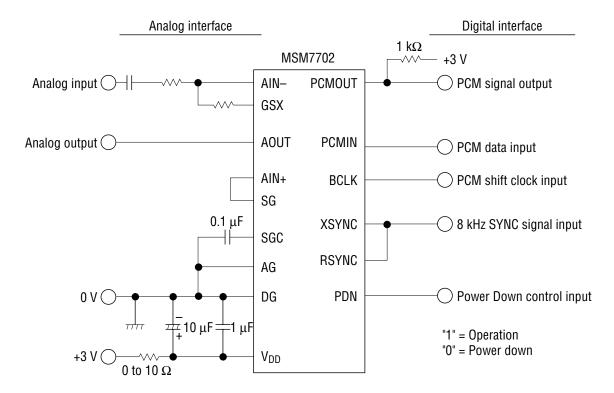
The analog output signal has a maximum amplitude of  $\pm 1.0$  V above and below the offset voltage level of  $V_{DD}/2$ .
