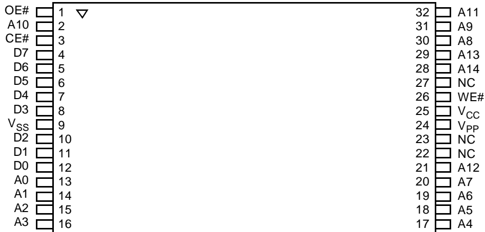
32-Pin TSOP—Reverse Pinout
