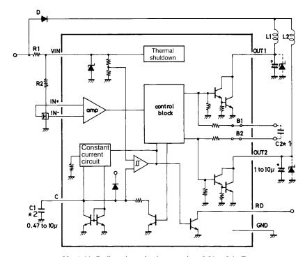
(Note) \*1: Radio noise reduction capacitor: 0.01 to 0.1  $\mu F\!.$
