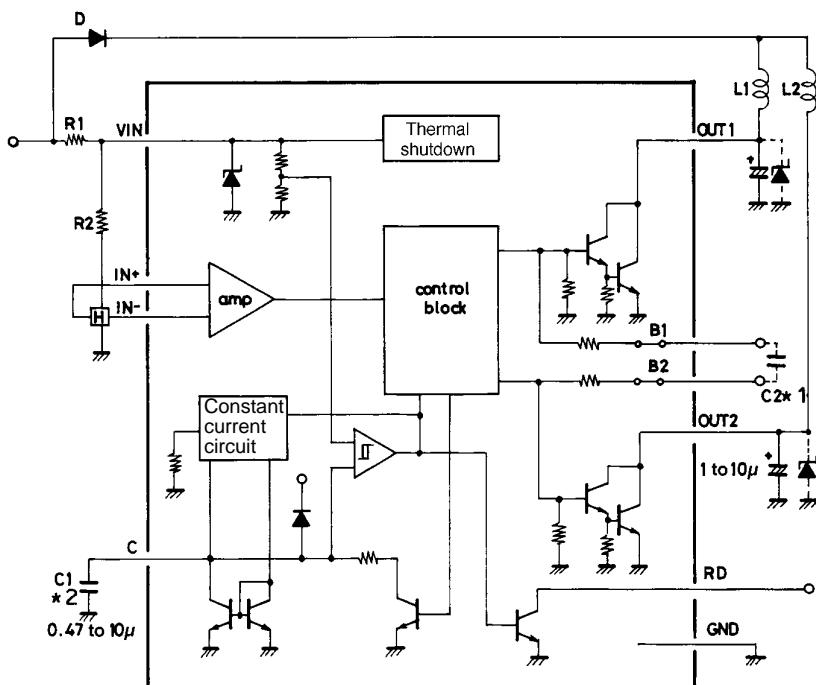
(Note) \*1: Radio noise reduction capacitor: 0.01 to 0.1 μF.
