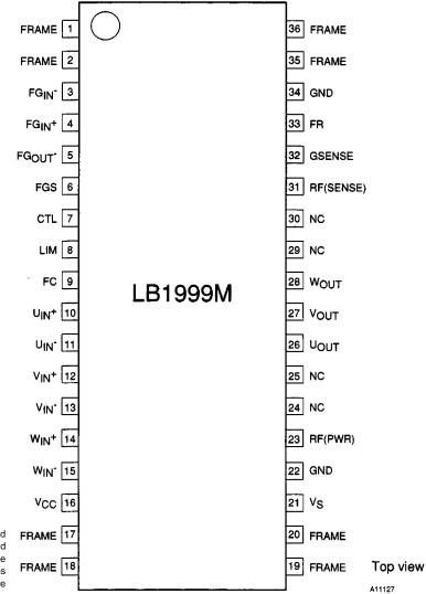
Note: Although the FRAME pins and the GND pins are not connected internally, the potentials of the GND pins and the FRAME pins externally be identical to assure ground potential stability.
