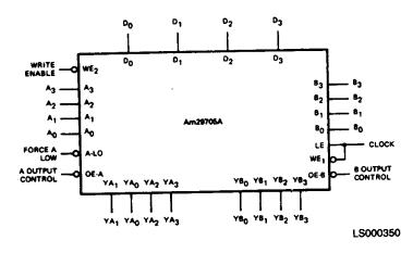
A 16-word by 4-bit two-port RAM with LE and WE<sub>1</sub> connected to make the device appear edge triggered. WE<sub>1</sub> and WE<sub>2</sub> are logically identical but are electrically slightly different. For
