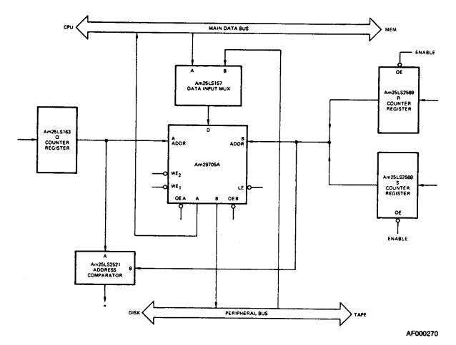
The Am29705A as a two-way interface buffer. Data may be passed between the main data bus and the peripheral data bus under I/O control. The two-port RAM allows data to be written into buffer storage from a peripheral device, using the B address port and the S counter register, while it is being read into main memory, using the A address port and the Q counter register. This simultaneous read/write capability facilitates DMA transfers because the CPU can ignore write requests
