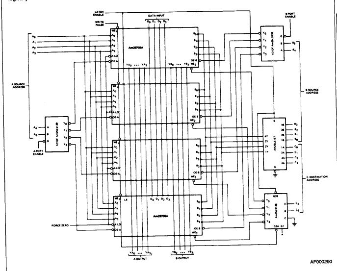
A 64-word by 4-bit three address memory. Data is read from the A address to the YA outputs and from the B address to the YB outputs while the latch enable is HIGH. When the latch enable goes LOW, the YA and YB data is held in the internal
