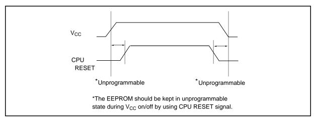
In addition, when  $V_{CC}$  is turned on or off, the input level of on control pins must be held as shown in the table below.
