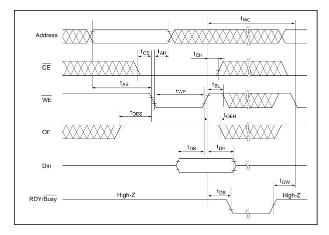
Byte Write Timing Waveform (1) (WE Controlled)
