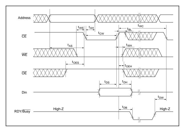
Byte Write Timing Waveform (2) (CE Controlled)
