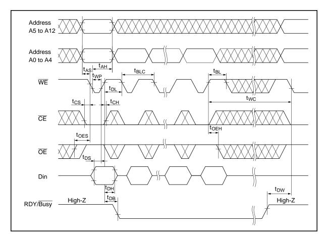
Page Write Timing Waveform (1) (WE Controlled)
