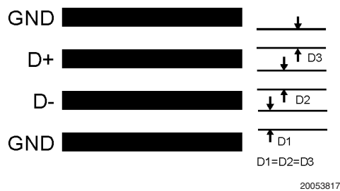
FIGURE 11. Ideal Diode Trace Layout
