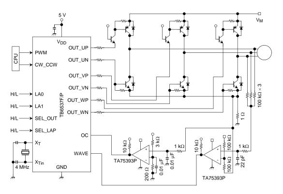
Note 1: Take enough care in designing output  $V_{DD}$  line and GND line to avoid short circuit between outputs,  $V_{DD}$  fault or GND fault which may cause the IC to break down.
