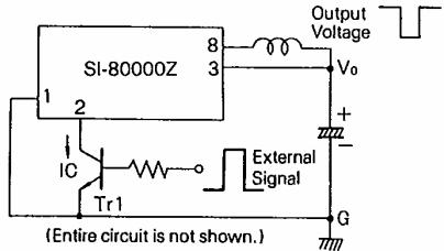
The output can be turned-off by a small signal transistor Tr1. Transistor size can be as small as  $P_c \approx 100\text{mW}$ .
