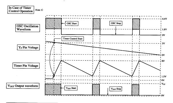
Note 2) In case of current limiting operation (CLM+ $\geq$ 0.2V and CLM- $\leq$ -0.2V),  $T_{OFF\ (max.)}$  control and timer control work. Note 3) Even during timer control operation, the OFF period of OSC ( $V_{OUT}$ ) is controlled by  $T_{OFF\ (max.)}$  control.
