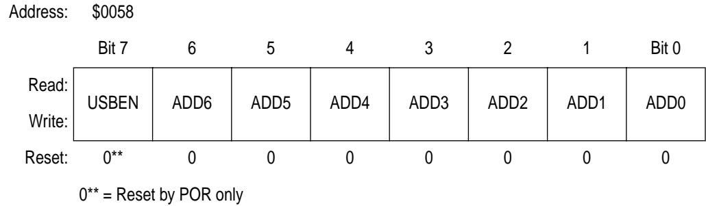
Figure 9-6. USB HUB Address Register (HADDR)
