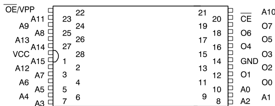
TSOP Top View Type 1
