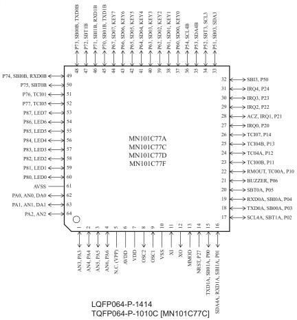
Note) N.C. serves as the VPP pin in the MN101CF77G, and cannot be used as a user pin.
