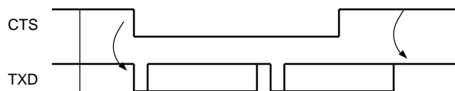
Figure 20-17. Transmitter Behavior when Operating with Hardware Handshaking
