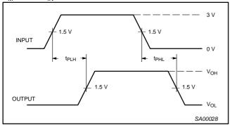
**Waveform 1. Input to Output Propagation Delays**
