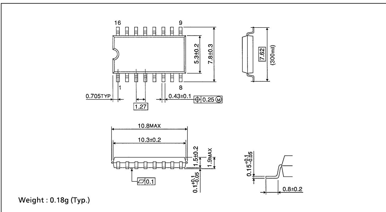
**SOP 16PIN (150mil BODY) PACKAGE DIMENSIONS (SOL16-P-150-1.27)**
