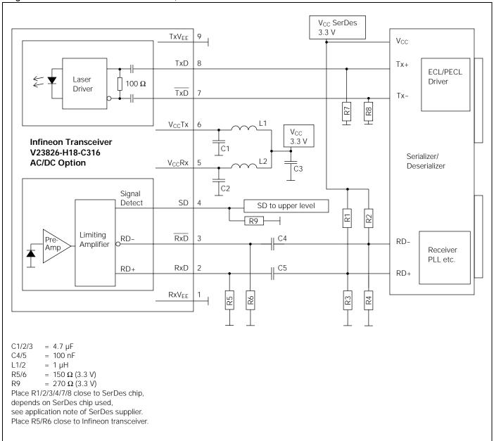
Values of R1/2/3/4 may vary as long as proper 50  $\Omega$  termination to V<sub>EE</sub> or 100  $\Omega$  differential is provided. The power supply filtering is required for good EMI performance. Use short tracks from the inductor L1/L2 to the module V<sub>CC</sub>Rx/V<sub>CC</sub>Tx. Further application notes for electrical interfacing are available upon request. Ask for Appnote 82.
