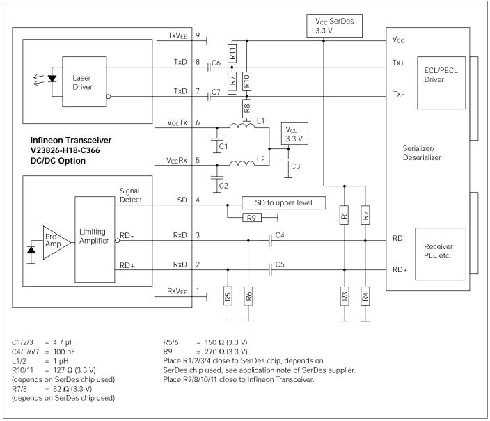
3.3 V-Transceivers can be directly connected to SerDes-Chips using standard PECL Termination network.
