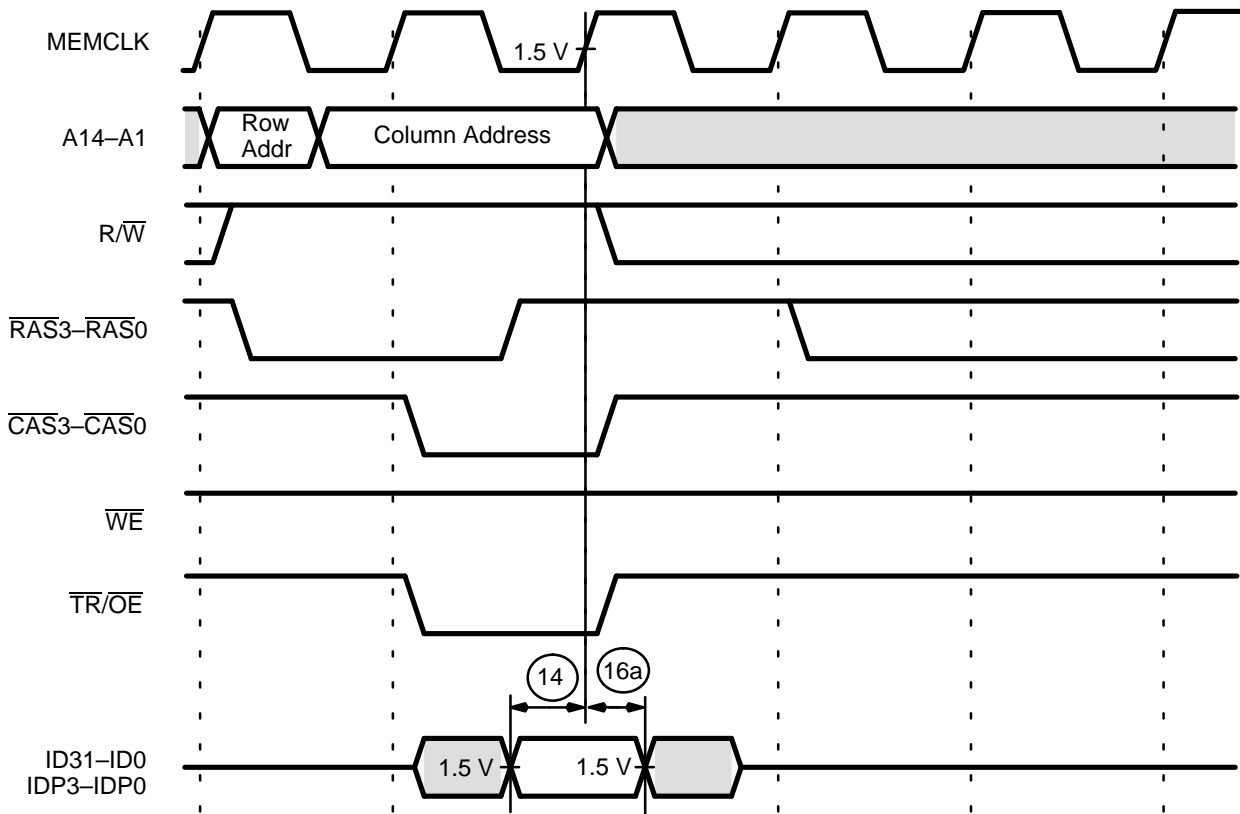
Figure 5. Simple 2/1 DRAM Read Cycle
