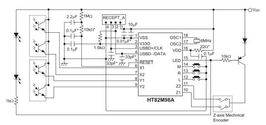
Note: Layout  $0.1\mu\text{F}$  capacitor,  $22\Omega$  resistor and  $0.01\mu\text{F}$  capacitor as close to VDD pin as possible.
