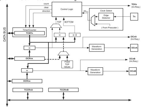
Figure 14-1. 8-bit Timer/Counter Block Diagram
