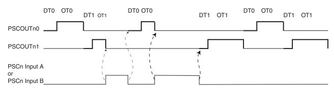
Used in Fault mode 6, PSCn Input A or PSCn Input B act indifferently on On-Time0/Dead-Time0 or on On-Time1/Dead-Time1.
