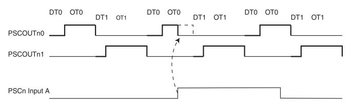
The output frequency is not modified by the occurence of significative edge of retriggering input.
