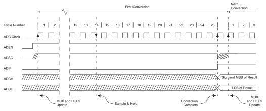
Figure 21-5. ADC Timing Diagram, Single Conversion
