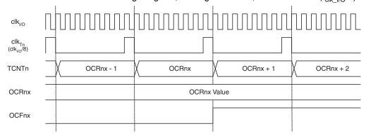
Figure 14-11 shows the setting of OCF0A and the clearing of TCNT0 in CTC mode and fast PWM mode where OCR0A is TOP.
