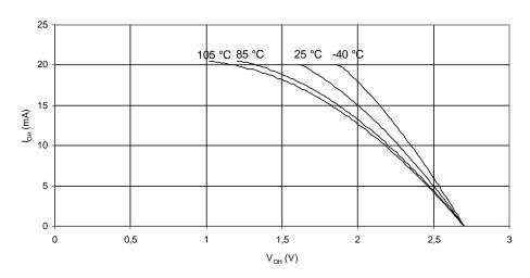
Figure 27-18. I/O Pin Sink Current vs. Output Voltage ( $V_{CC} = 5V$ )
