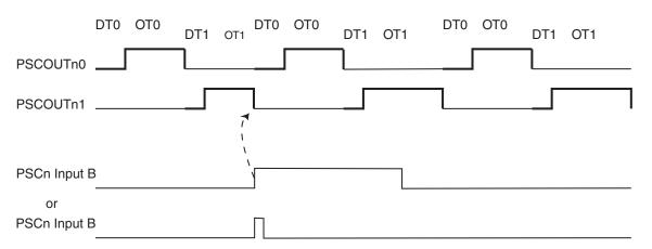
The output frequency is modulated by the occurrence of significative edge of retriggering input.
