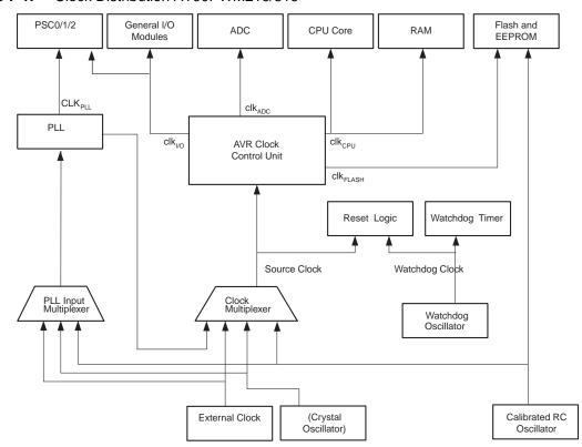
Figure 7-1. Clock Distribution AT90PWM216/316
