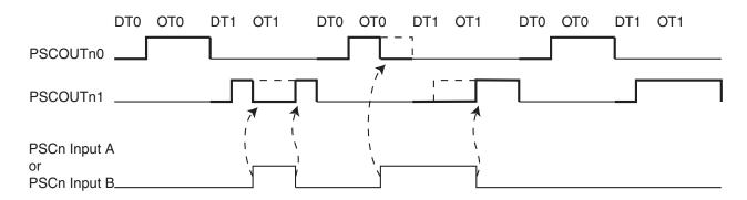
Figure 16-27. PSC behaviour versus PSCn Input A or Input B in Fault Mode 4
