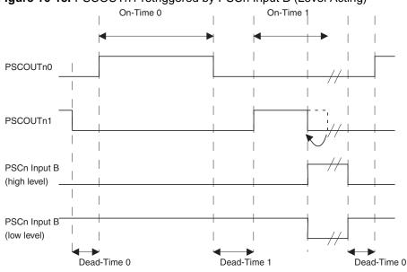
Figure 16-18. PSCOUTn1 retriggered by PSCn Input B (Level Acting)
