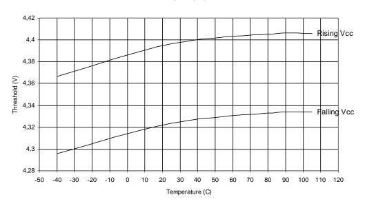
Figure 27-31. BOD Thresholds vs. Temperature (BODLEVEL Is 2.7V)
