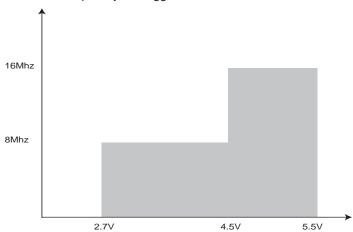
Figure 26-2. Maximum Frequency vs.  $V_{CC}$ , AT90PWM216/316
