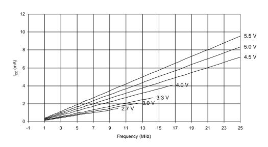
Figure 27-7. IIdle Supply Current vs. V<sub>CC</sub> (Internal RC Oscillator, 8 MHz)
