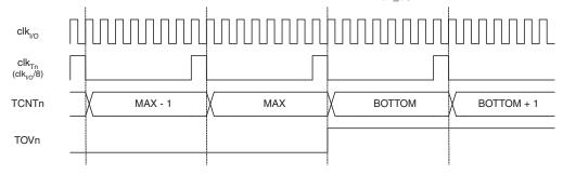
Figure 14-10 shows the setting of OCF0B in all modes and OCF0A in all modes except CTC mode and PWM mode, where OCR0A is TOP.
