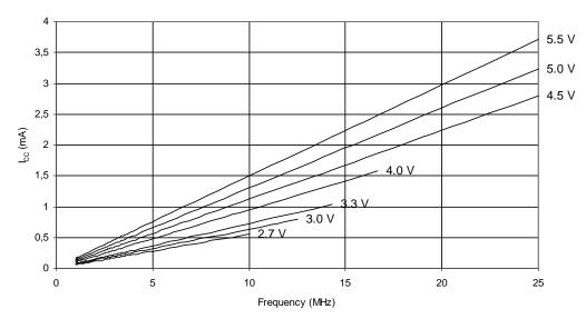
**Figure 27-47.** Reset Supply Current vs. V<sub>CC</sub> (Clock Stopped, Excluding Current through the Reset Pull-up)
