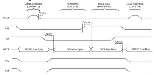
Note: 1. The timing requirements shown in Figure 25-7 (i.e., t<sub>DVXH</sub>, t<sub>XHXL</sub>, and t<sub>XLDX</sub>) also apply to reading operation.
