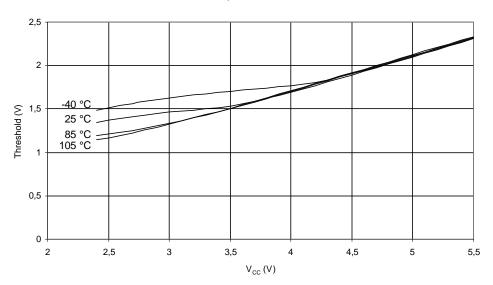
Figure 27-24. Reset Input Threshold Voltage vs.  $V_{CC}$  (VIL, Reset Pin Read As '0') RESET INPUT THRESHOLD VOLTAGE vs.  $V_{CC}$  VIL, RESET PIN READ AS '0'
