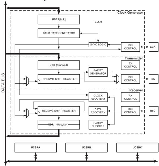
Note: 1. Refer to Pin Configurations3, Table 11-9 on page 73, and Table 11-7 on page 71 for USART pin placement.
