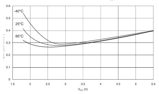
Figure 27-23. Reset Input Threshold Voltage vs.  $V_{CC}$  (VIH, Reset Pin Read As '1')
