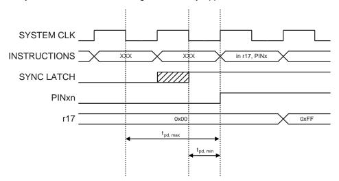
Figure 11-3. Synchronization when Reading an Externally Applied Pin value
