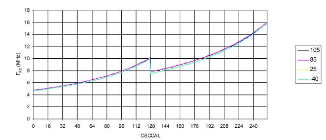
Figure 27-39. Calibrated 8 MHz RC Oscillator Frequency vs. Osccal Value
