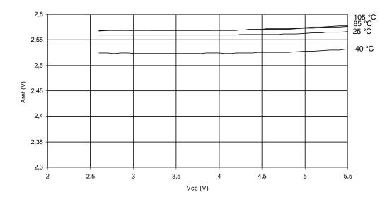
Figure 27-35. AREF Voltage vs. Temperature
