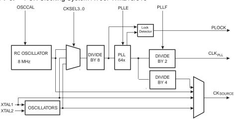
Figure 7-3. PCK Clocking System AT90PWM216/316
