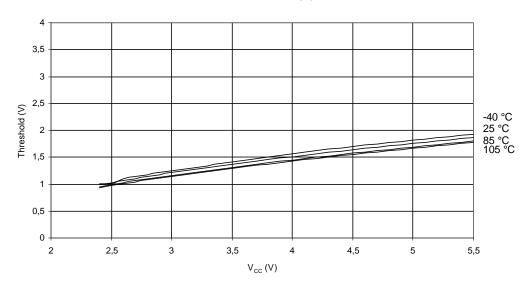
Figure 27-28. PE0 Input Threshold Voltage vs.  $V_{CC}$  (PE0 Pin Read As '1')
