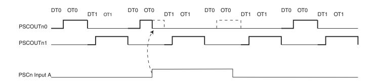
The output frequency is not modified by the occurence of significative edge of retriggering input.
