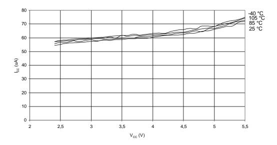
Figure 27-44. Programming Current vs.  $V_{CC}$
