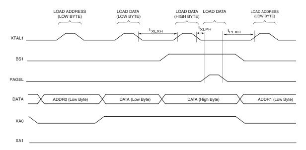
Note: 1. The timing requirements shown in Figure 26-5 (i.e., t<sub>DVXH</sub>, t<sub>XHXL</sub>, and t<sub>XLDX</sub>) also apply to loading operation.
