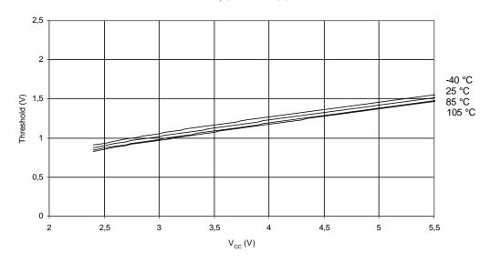
Figure 27-22. I/O Pin Input HysteresisVoltage vs.  $V_{CC}$  I/O PIN INPUT HYSTERESIS vs.  $V_{CC}$
