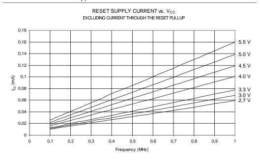
**Figure 27-46.** Reset Supply Current vs. V<sub>CC</sub> (1 - 24 MHz, Excluding Current through the Reset Pull-up)
