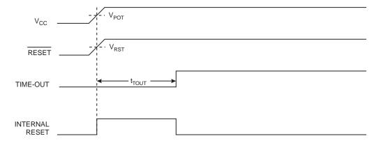
Figure 9-3. MCU Start-up, RESET Extended Externally
