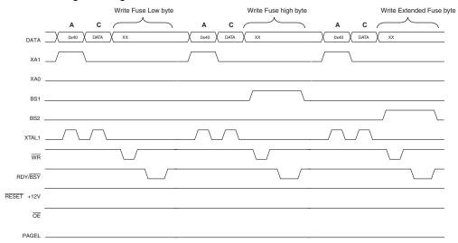
Figure 25-5. Programming the FUSES Waveforms
