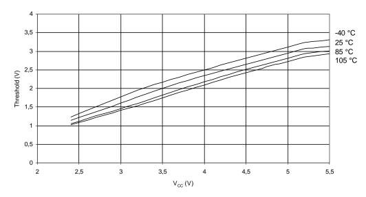
Figure 27-27. XTAL1 Input Threshold Voltage vs. V<sub>CC</sub> (XTAL1 Pin Read As '0')
