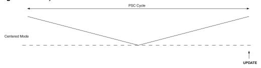
Ramps illustrate the output of the PSC counter included in the waveform generators. Centered Mode is like a one ramp mode which count down up and down.
