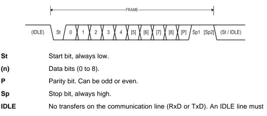
The frame format used by the USART is set by the UCSZ2:0, UPM1:0 and USBS bits in UCSRB and UCSRC. The Receiver and Transmitter use the same setting. Note that changing the setting of any of these bits will corrupt all ongoing communication for both the Receiver and Transmitter.
