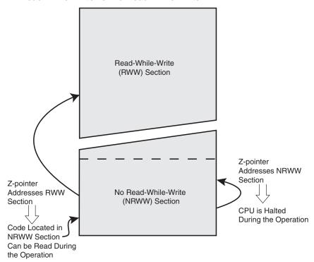
Figure 24-1. Read-While-Write vs. No Read-While-Write
