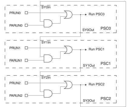
Figure 16-38. PSC Run Synchronization
