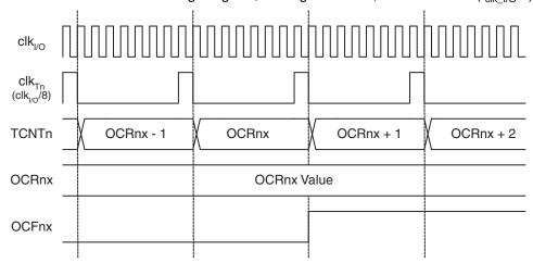
Figure 15-11. Timer/Counter Timing Diagram, Setting of OCFnx, with Prescaler (f<sub>clk I/O</sub>/8)
