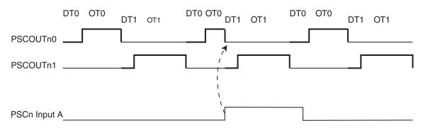
The output frequency is modulated by the occurence of significative edge of retriggering input.
