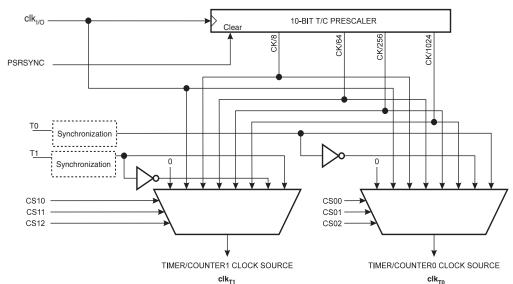
Figure 13-2. Prescaler for Timer/Counter0 and Timer/Counter1<sup>(1)</sup>
