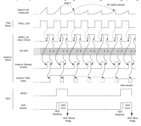
**Figure 21-16.** Amplifier synchronization timing diagram: behavior when ADSC is set when theamplifier output is changing.
