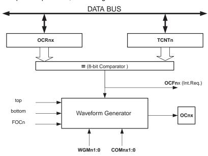
Figure 14-3. Output Compare Unit, Block Diagram
