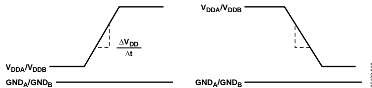
Figure 13. Transient Immunity Waveforms—Output Supplies
