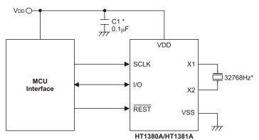
Note: \* In order to obtain the correct frequency, it is recommended to use a crystal with a load capacitance of 9.0pF. It is not recommended to connect load capacitors to the X1 and X2 pins. If the power line is noisy, it is recommended to add R1 and C1 for filtering out noise.
