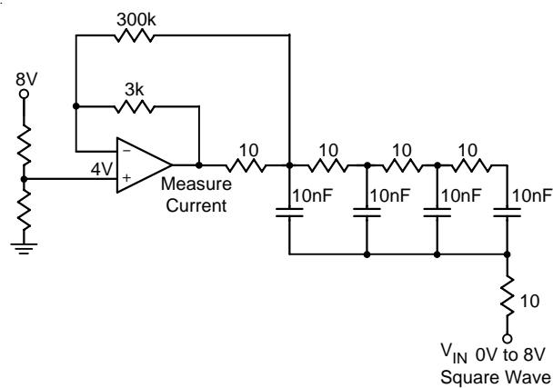
Figure 3. V-com Test Circuit
