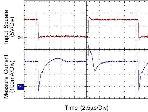
Figure 4. Scope Photo of the V-com Peak Current
