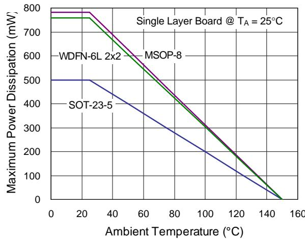
Figure 2. Derating Curves for the RT9133A/B Package
