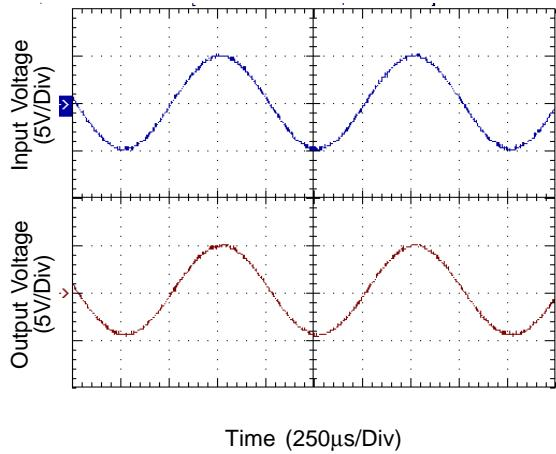
Figure 1. Operation with Rail-to-Rail Input and Output
