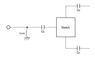
• CB are DC blocking capacitors external to the device.
