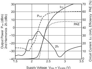
Condition: Vcc1 = Vcc2 = Vbias + Venable = Vcont = 3.0 V, Pin = -20 dBm, with external input and output matching circuit
