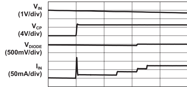
Load Switch to Charge Pump (1.5X Mode, 4x30mA Load)
