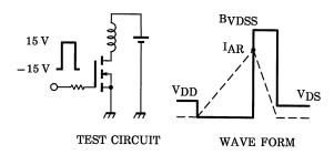
$$\begin{aligned} &R_G = 25~\Omega \\ &V_{DD} = 90~V,~L = 594~mH \end{aligned} \qquad E_{AS} = \frac{1}{2} \cdot L \cdot I^2 \cdot \left( \frac{BVDSS}{BVDSS - V_{DD}} \right)$$
