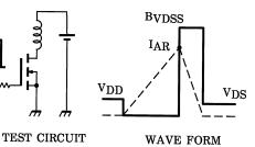
$R_G = 25 \Omega$  $V_{\rm DD}$  = 90 V, L = 4.08 mH
