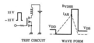
$$\begin{aligned} R_G &= 25 \ \Omega \\ V_{DD} &= 25 \ V, \ L = 4.2 \ mH \end{aligned} \qquad E_{AS} = \frac{1}{2} \cdot L \cdot I^2 \cdot \left( \frac{BVDSS}{BVDSS - V_{DD}} \right)$$
