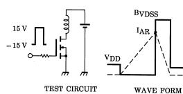
$$\begin{aligned} R_G &= 25~\Omega \\ V_{DD} &= 25~V,~L = 530~\mu H \end{aligned} \qquad E_{AS} &= \frac{1}{2} \cdot L \cdot I^2 \cdot \left( \frac{Bv_{DSS}}{Bv_{DSS} - V_{DD}} \right) \end{aligned}$$
