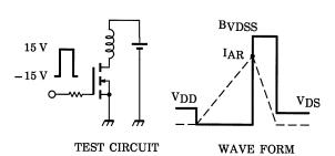
$$\begin{aligned} &R_G = 25~\Omega \\ &V_{DD} = 90~V,~L = 28.8~mH \end{aligned} \qquad E_{AS} = \frac{1}{2} \cdot L \cdot I^2 \cdot \left( \frac{BVDSS}{BVDSS - V_{DD}} \right) \end{aligned}$$
